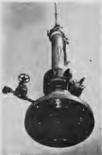
FULLY-EQUIPPED Mueller Hot Tap machines cost about $7000 each. Much time is saved in tapping product lines with the hot tap units. MUELLER HOT Tap mashien cu armacion completo ta costa como $7000. E tempo cu nan ta spaar compania ta hustifica nan costo.
